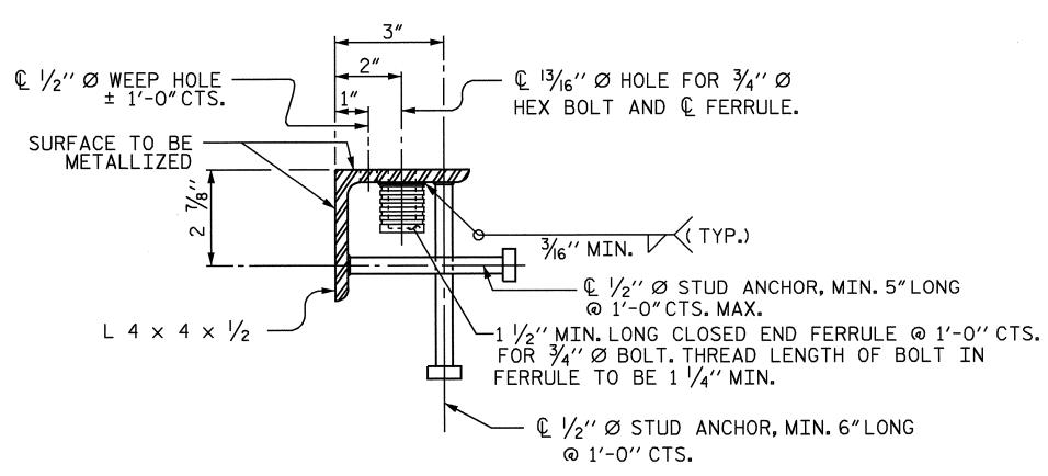
TYPICAL SECTION OF BASE ANGLE ASSEMBLY
