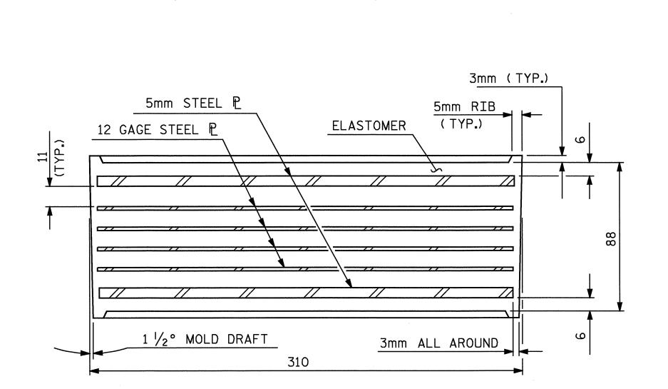
TYPICAL SECTION OF ELASTOMERIC BEARING
