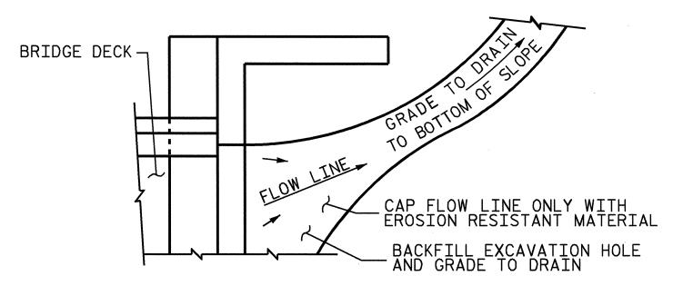
NOTE: IF THE APPROACH SLAB IS NOT CONSTRUCTED IMMEDIATELY AFTER THE BACKFILLING OF THE END BENT EXCAVATION, GRADE TO DRAIN TO THE BOTTOM OF THE SLOPE AND PROVIDE EROSION RESISTANT MATERIAL, SUCH AS FIBERGLASS ROVING OR AS DIRECTED BY THE ENGINEER TO PREVENT SOIL EROSION AND TO PROTECT THE AREA ADJACENT TO THE STRUCTURE. THE CONTRACTOR WILL BE REQUIRED TO REMOVE THESE MATERIALS PRIOR TO CONSTRUCTION OF THE APPROACH SLAB.
