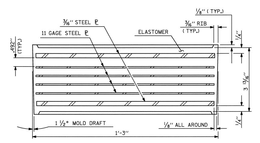
TYPICAL SECTION OF ELASTOMERIC BEARING
