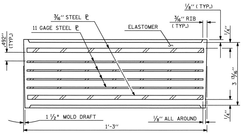
TYPICAL SECTION OF ELASTOMERIC BEARING
