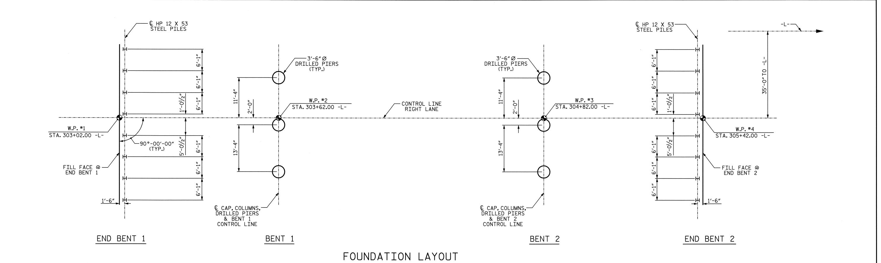
PILE LOCATION IS TO © PILE. ALL PILES AT END BENTS ARE HP 12 X 53 STEEL PILES BENTS 1 & 2 HAVE DRILLED PIERS.
