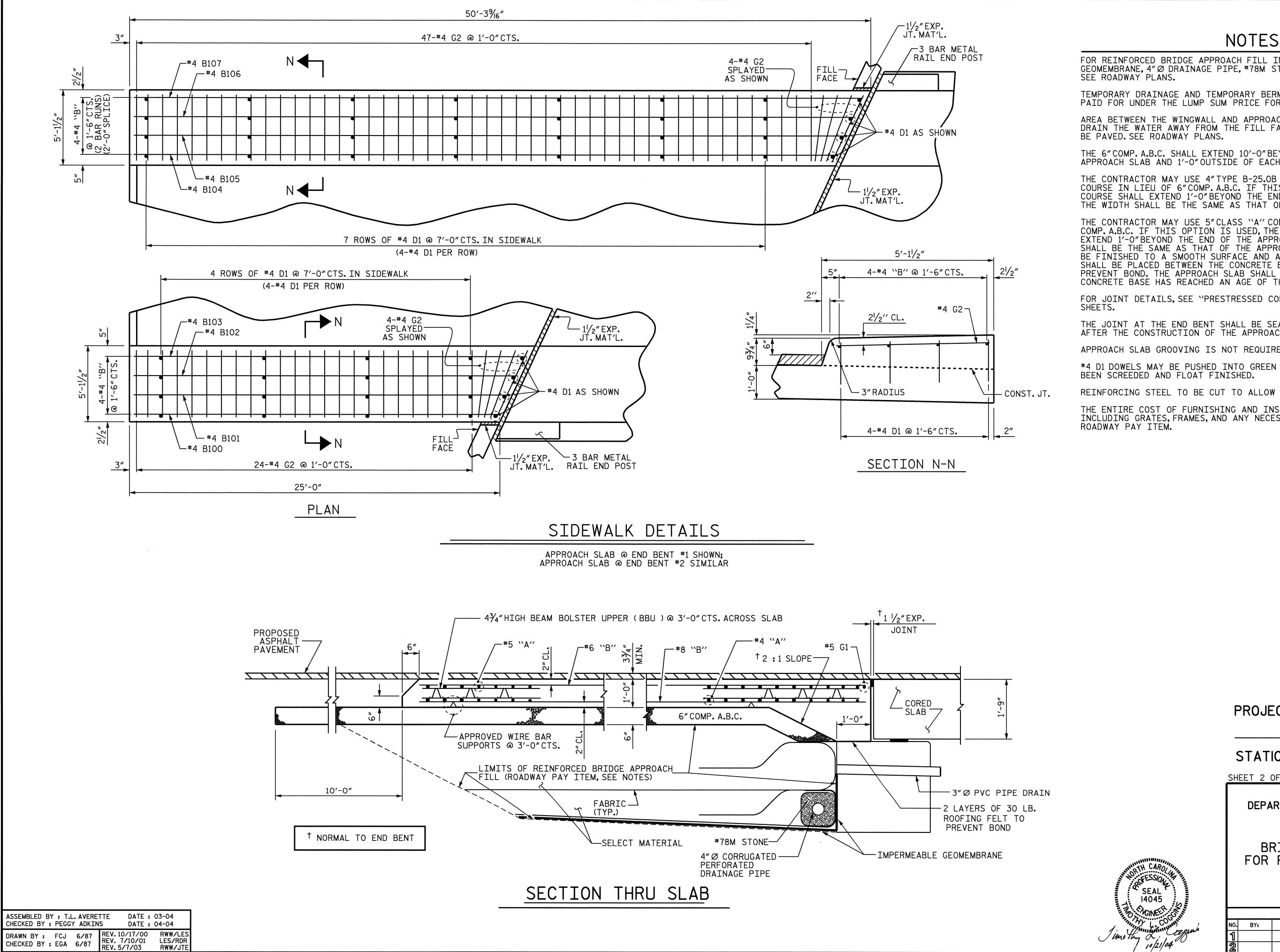
FOR REINFORCED BRIDGE APPROACH FILL INCLUDING FABRIC, IMPERMEABLE GEOMEMBRANE, 4" Ø DRAINAGE PIPE, #78M STONE, AND SELECT MATERIAL,
