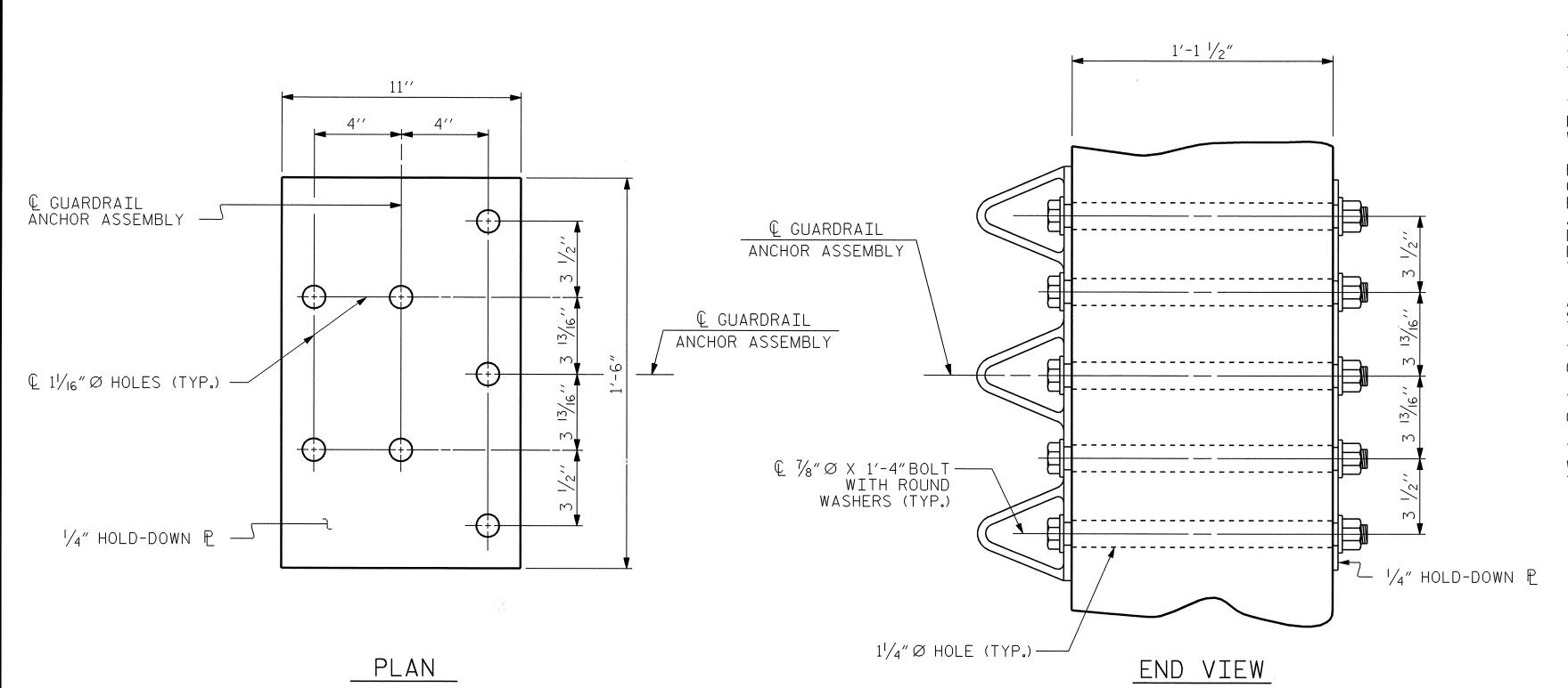
GUARDRAIL ANCHOR ASSEMBLY DETAILS
