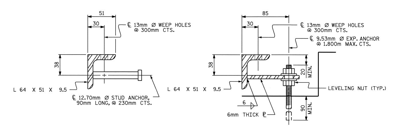
ARMORED JOINT ANCHOR ASSEMBLY DETAILS
