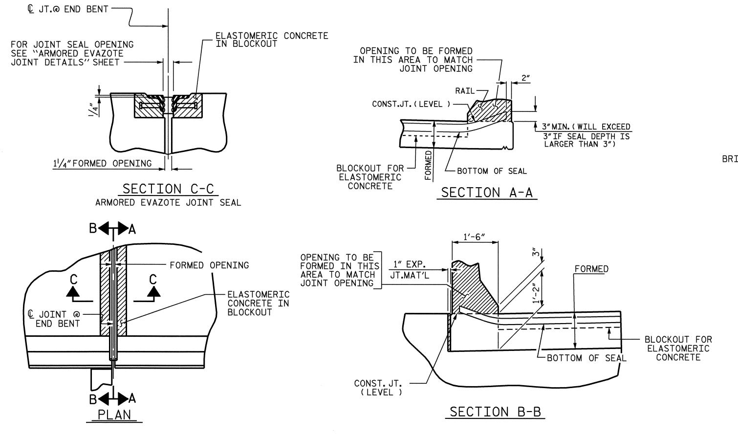
JOINT SEAL DETAILS @ END BENT
