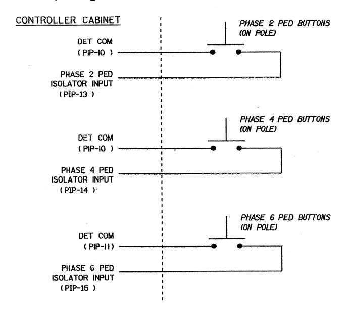
NOTE: MAKE SURE PED ISOLATOR CIRCUIT IS PRESENT IN CONTROLLER/CABINET ASSEMBLY.
