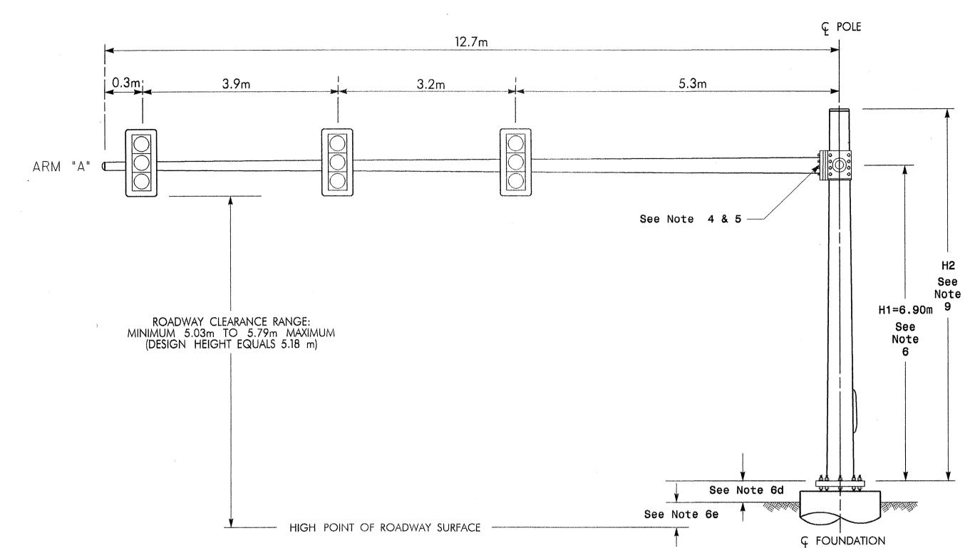
Design Loading for METAL POLE NO. 7, MAST ARM A
