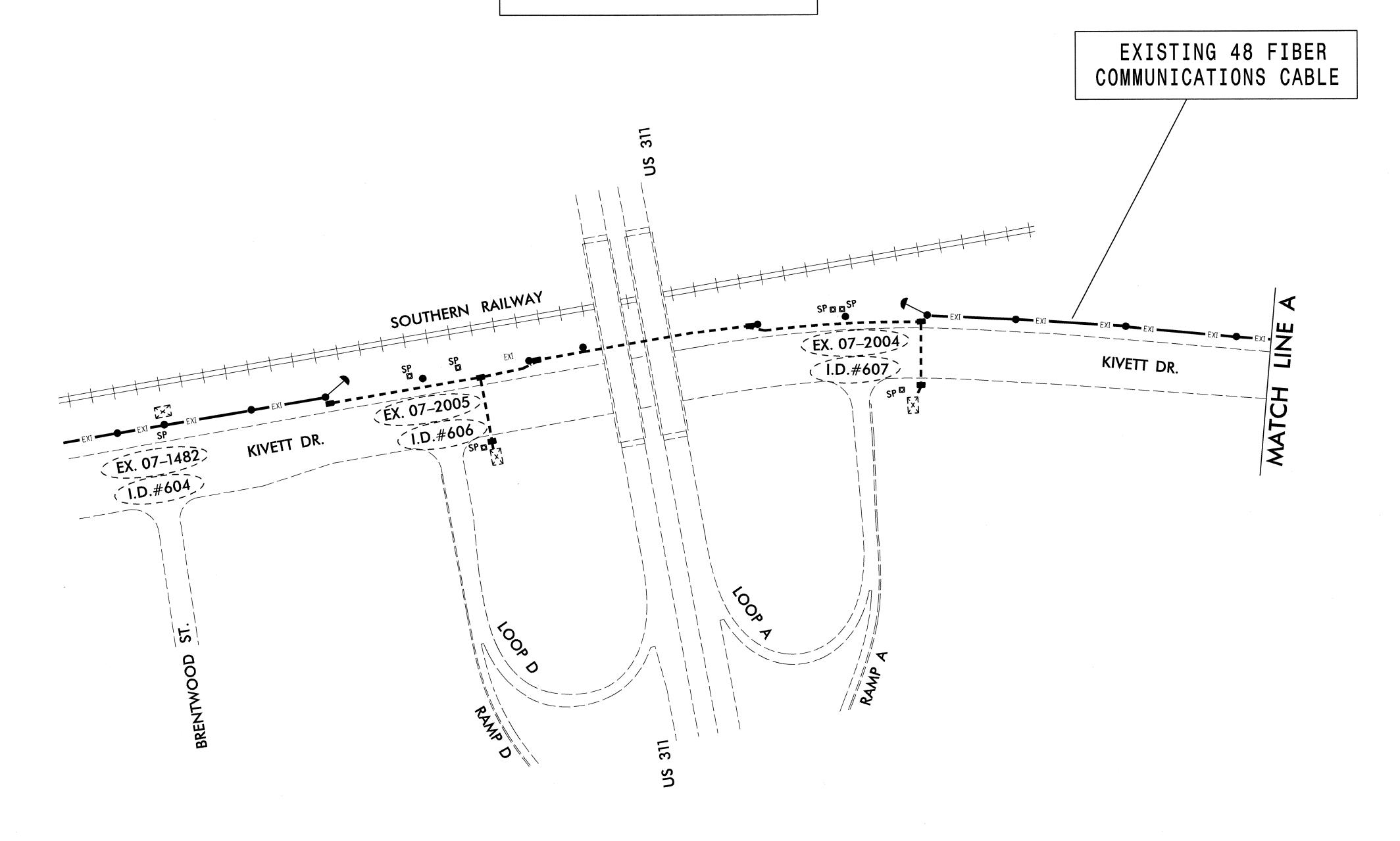
ALL NCDOT COMMUNICATIONS CABLE ATTACHMENT POINTS ARE 1 METER (40 INCHES) BELOW POWER (FRONT SIDE OF POLE) UNLESS OTHERWISE NOTED.
