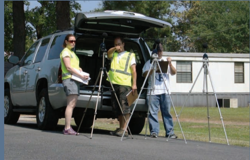
Noise readings were taken at many locations along the DSAs. Along with traffic count data, these readings were used to establish a database of existing noise levels.
