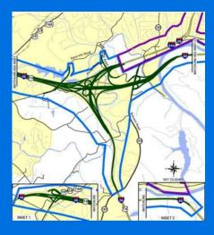
Provides two flyover ramps and two loop ramps at the I-26/I-40/I-240 interchange along with collector-distributor roadways in both directions along I-40 and in the eastbound direction along I-26.
