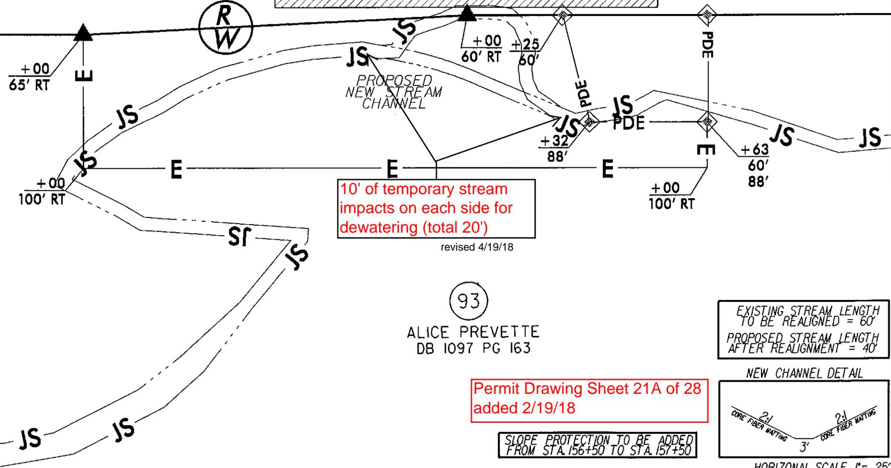
10' of temporary stream impacts on each side for dewatering (total 20')
