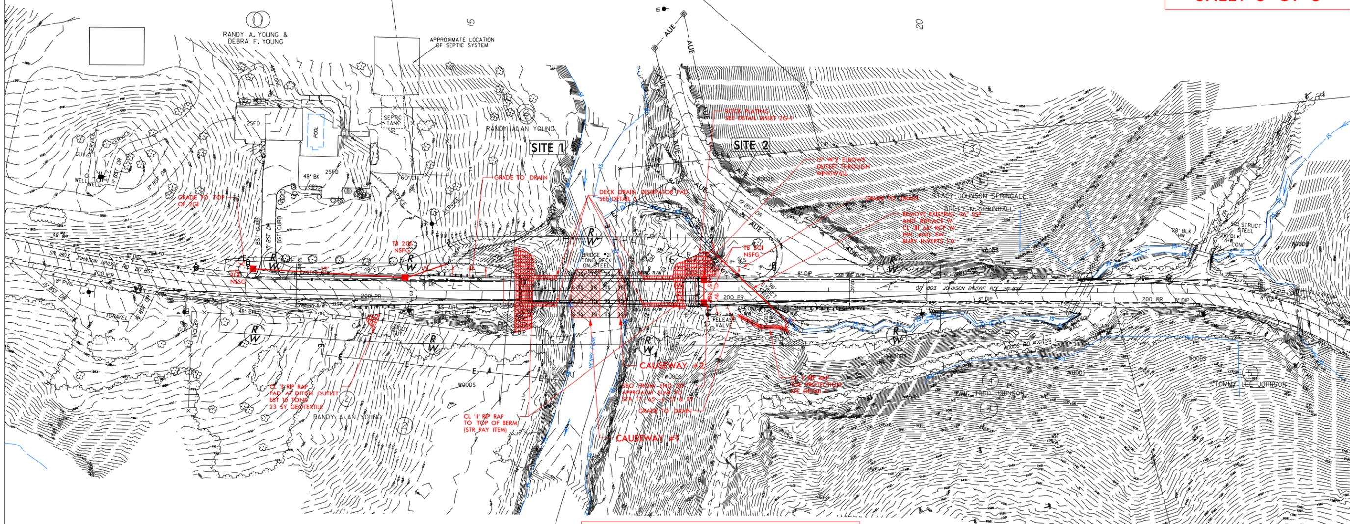
THE DRAWING DEPICTS THE TOTAL AREA BEING IMPACTED BY THE CONSTRUCTION OF THE TEMPORARY CAUSEWAYS. HOWEVER, THE CAUSEWAYS WILL BE CONSTRUCTED IN TWO PHASES AND NEITHER PHASE WILL ENCOMPASS MORE THAN HALF OF THE STREAM CHANNEL.
