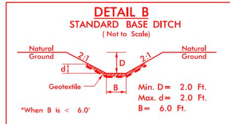
Type of Liner = Class I Rip-Rap FROM STA. 17+05 TO STA. 17+45 -L- Lt Excavation: Est. 90 cu yds Rip Rap: Est. 15 ton CII Geotextile: Est. 700 sq. ft.
