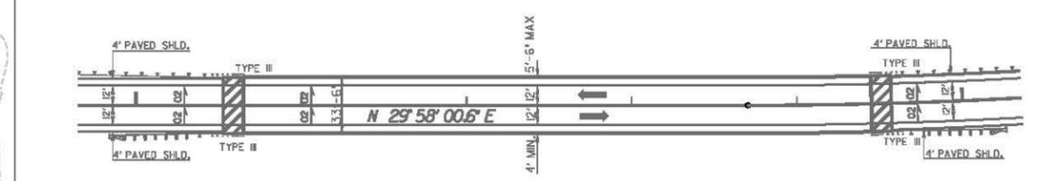
NOTE: DECK DRAINS ARE TO BE INSTALLED @ 3' CENTERS FOR THE FOLLOWING STATION RANGE:
