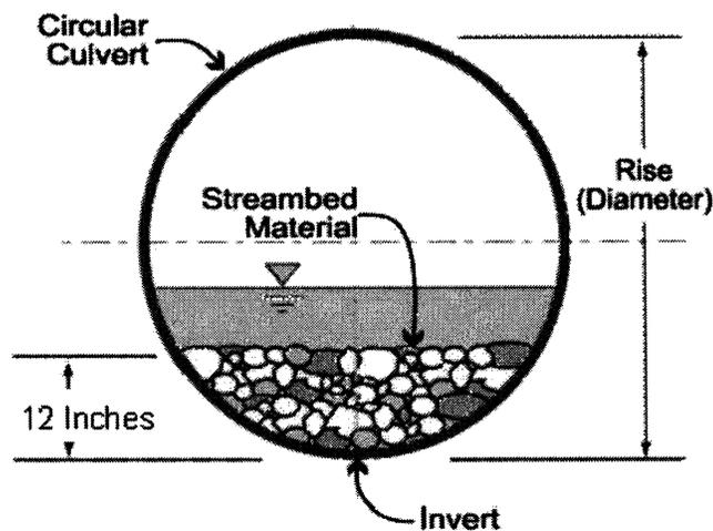
In all other counties: Culverts greater than 48 inches in diameter will be buried at least one foot below the bed of the stream. Culverts 48 inches in diameter or less shall be buried or placed on the stream bed as practicable and appropriate to maintain aquatic passage, and every effort shall be made to maintain the existing channel slope. The bottom of the culvert must be placed at a
