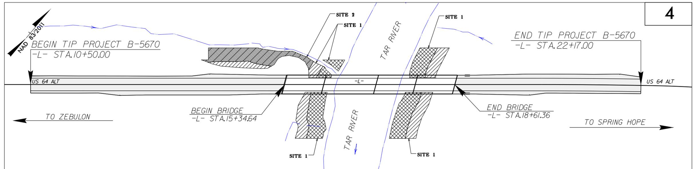
A DESIGN EXCEPTION WILL BE REQUIRED FOR MAXIMUM GRADE, SAG VERTICAL CURVE AND VERTICAL STOPPING SIGHT DISTANCE. THIS PROJECT IS NOT WITHIN MUNICIPAL BOUNDARIES. CLEARING ON THIS PROJECT SHALL BE PERFORMED TO THE LIMITS ESTABLISHED BY METHOD III.
