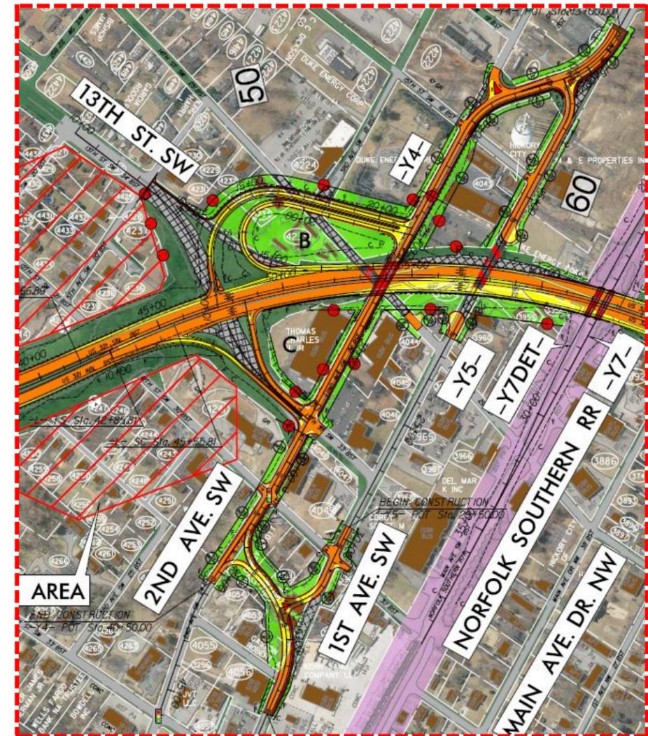
Figure 3: (Recommended) 2<sup>nd</sup> Avenue SW interchange design, January 2018
