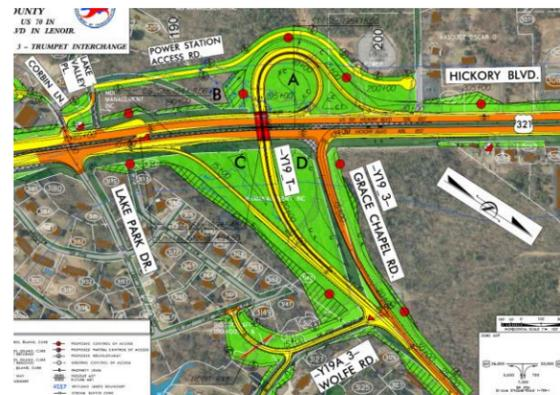
Figure 6: Trumpet interchange design, July 2016 public hearing (plus Wolfe Rd connector)
