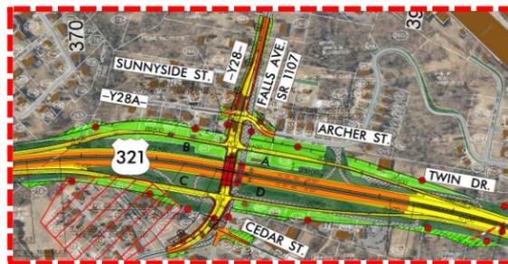
Figure 19: (Recommended) Tight diamond interchange design, January 2018
