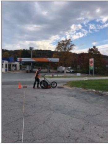
Photo 1. Collecting GPR grid data at Parcel #015.
