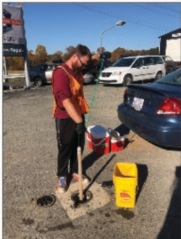
Photo 3. Bailing water from MW-9 in order to collect water samples.
