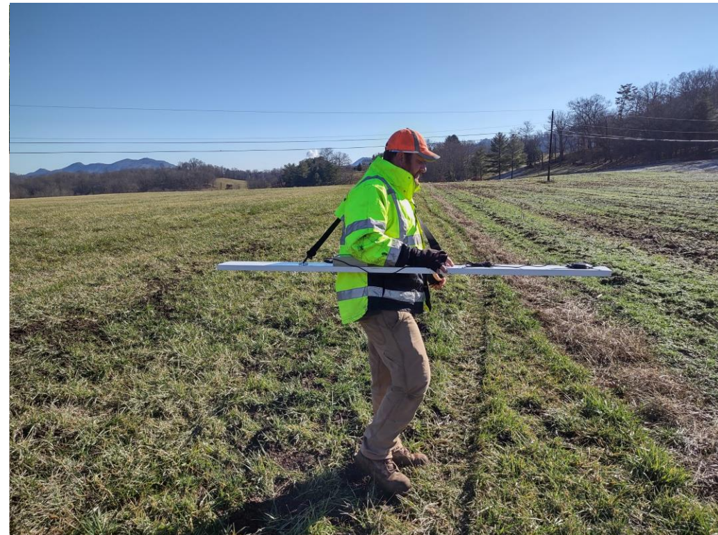
C. GEM2 multi-frequency EM instrument used to collect EM data at site (photograph from different project).
