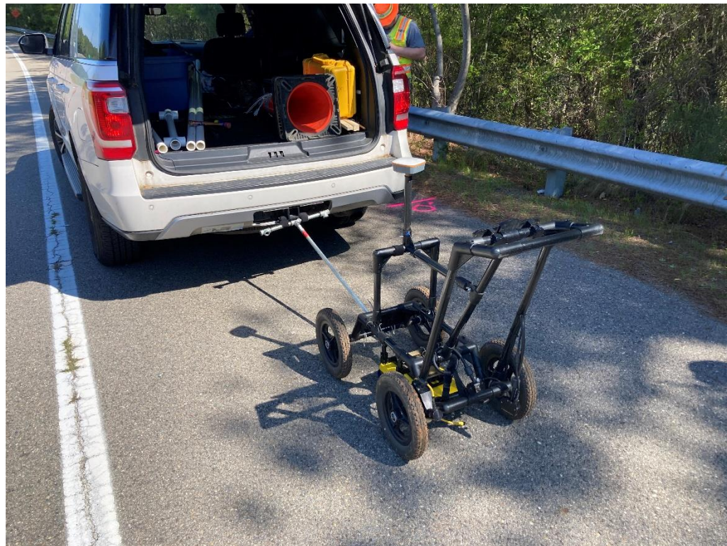
B. Noggin GPR cart with 500 MHz antenna set up to tow behind vehicle. Data also was collected by pushing the GPR cart by hand.
