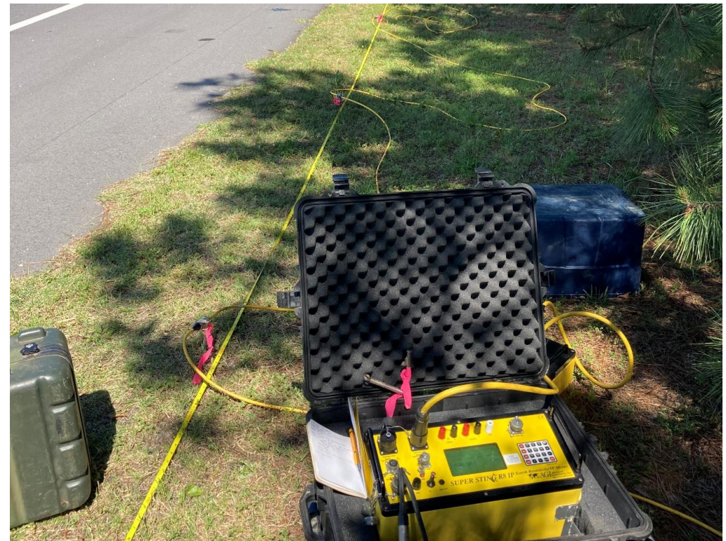
D. Electrical Resistivity Imaging (ERI) being collected on outside shoulder of northbound lane using R8 Supersting resistivity system with 56 electrodes.
