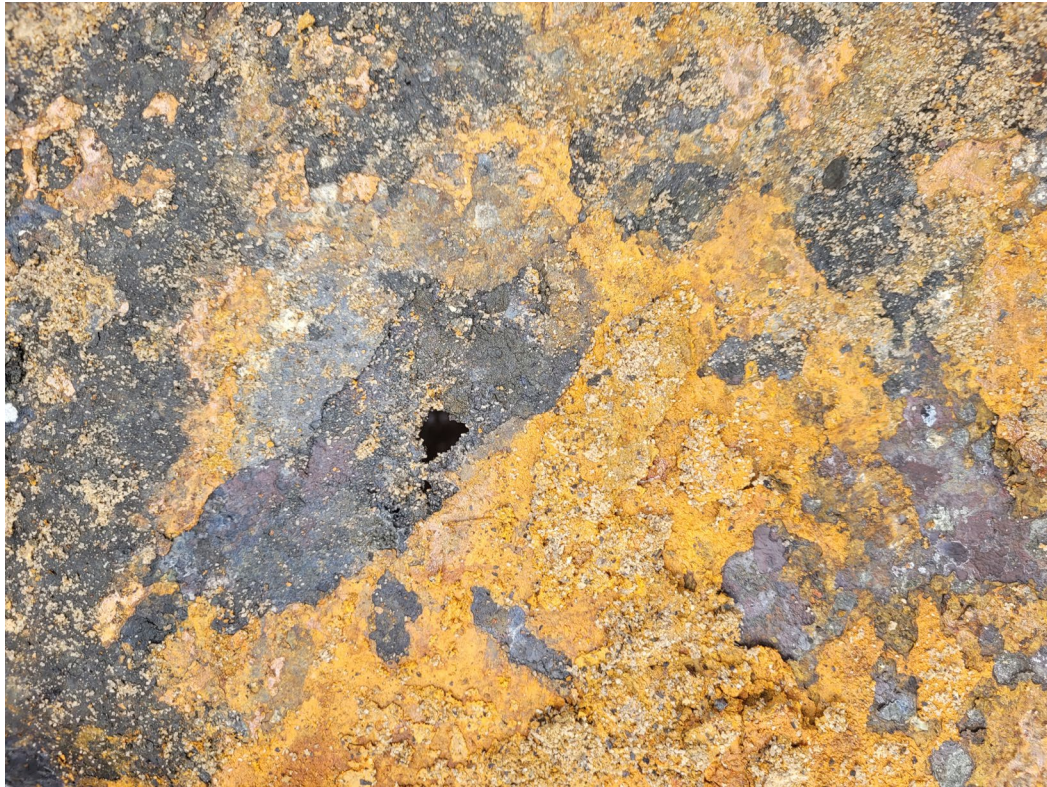
Photo 17 – View of tank with severe rusting and through hole (typical) on 1/16/2025.
