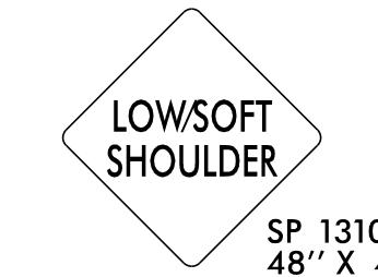
PLACE INITIALLY AT THE CONSTRUCTION LIMITS AND SPACED 1 MILE APART
