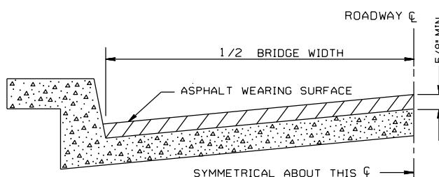
FOR BRIDGES WITH FLOOR DRAINS, CARE SHALL BE EXERCISED IN PLACING THE WEARING SURFACE AROUND FLOOR DRAINS SO AS NOT TO HINDER EFFECTIVE DRAINAGE. ALL DRAINS SHALL BE LEFT OPEN.
