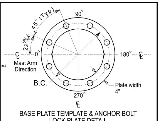
LOCK PLATE DETAIL For 8 Bolt Base Plate
