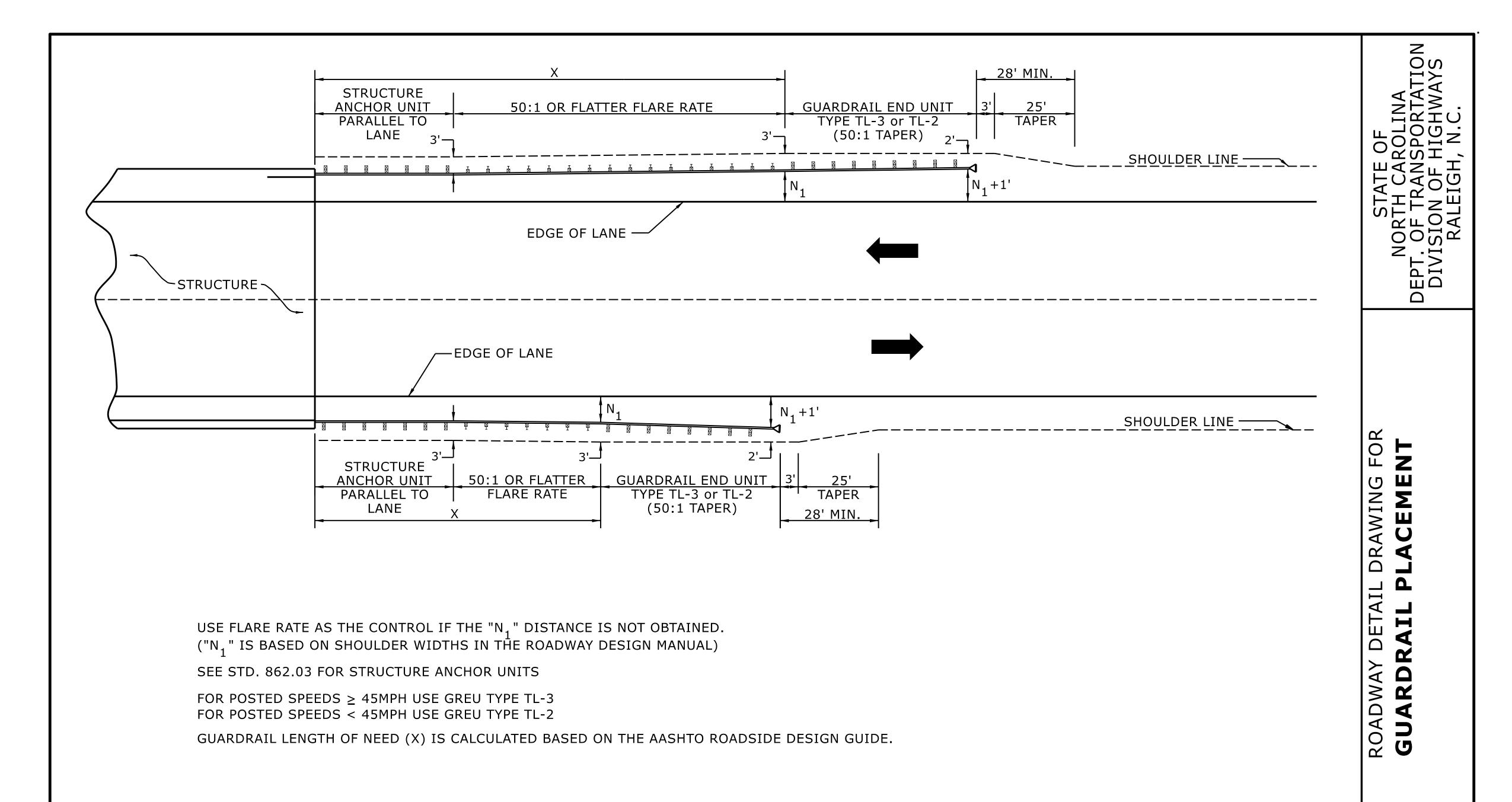
LENGTHS AND OFFSETS FOR PROPOSED GUARDRAIL AT TWO LANE - TWO WAY LOCATIONS
