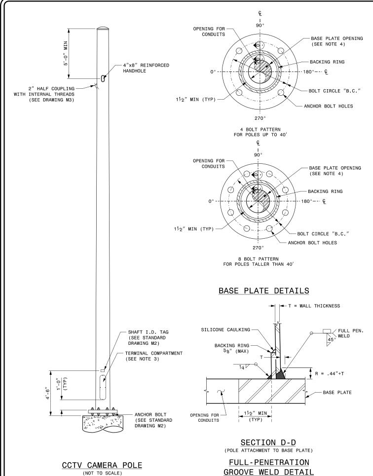
GROOVE WELD DETAIL
