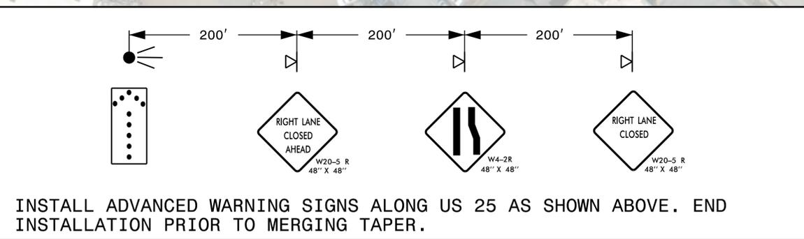
INSTALL ADVANCED WARNING SIGNS ALONG US 25 AS SHOWN ABOVE. END INSTALLATION PRIOR TO MERGING TAPER.
