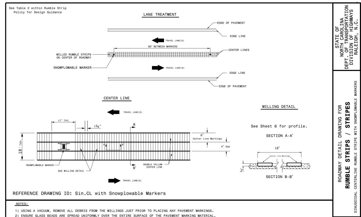
3) INSTALL SNOWPLOWABLE MARKERS AT APPROXIMATELY 80' INCREMENTS. DO NOT MILL RUMBLE STRIPS IN SECTION WHERE SNOWPLOWABLE MARKERS ARE INSTALLED.
