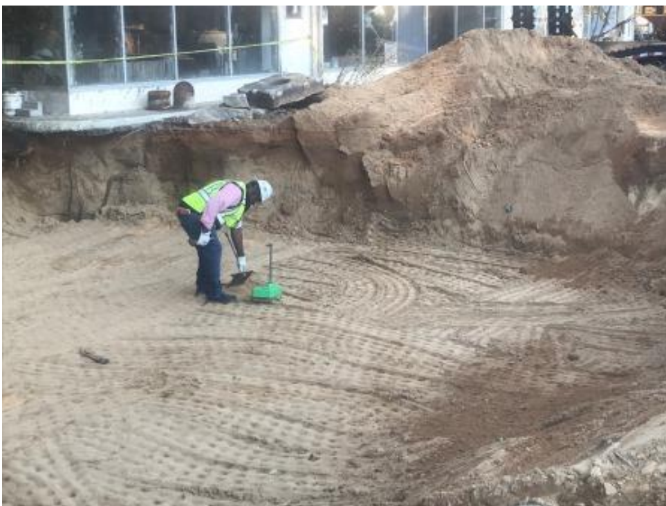
Photograph 11: Ken Thorpe performing compaction testing at four feet below ground surface.
