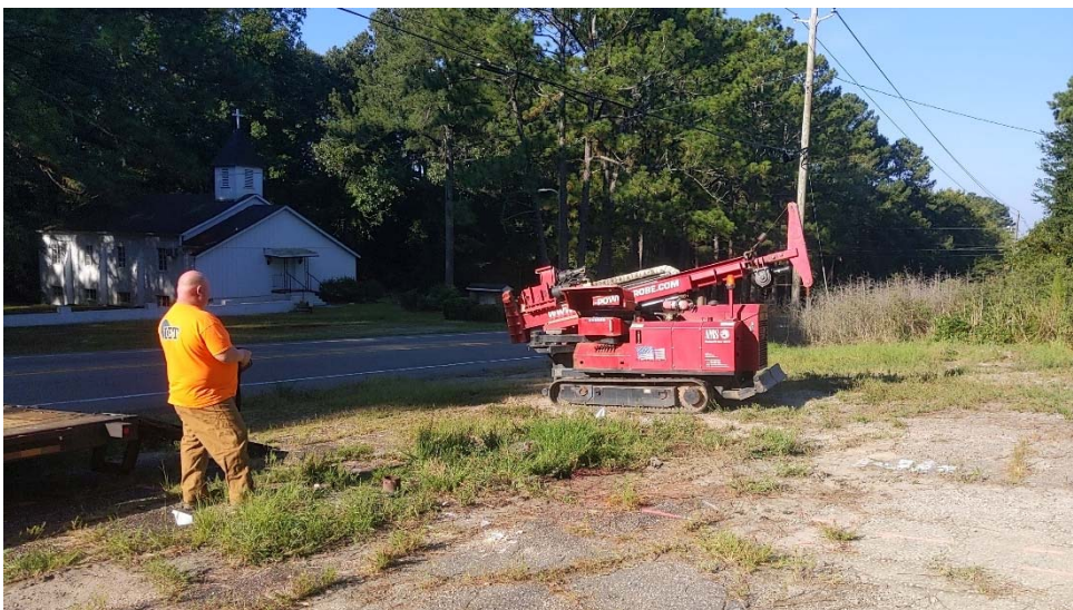
Photograph 4: View of IET maneuvering direct- push rig to collect soil samples, facing southwest.
