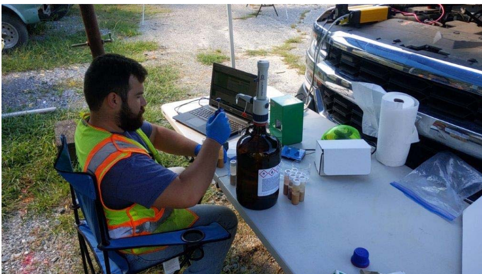
Photograph 5: View of on-Site UVF analysis setup.
