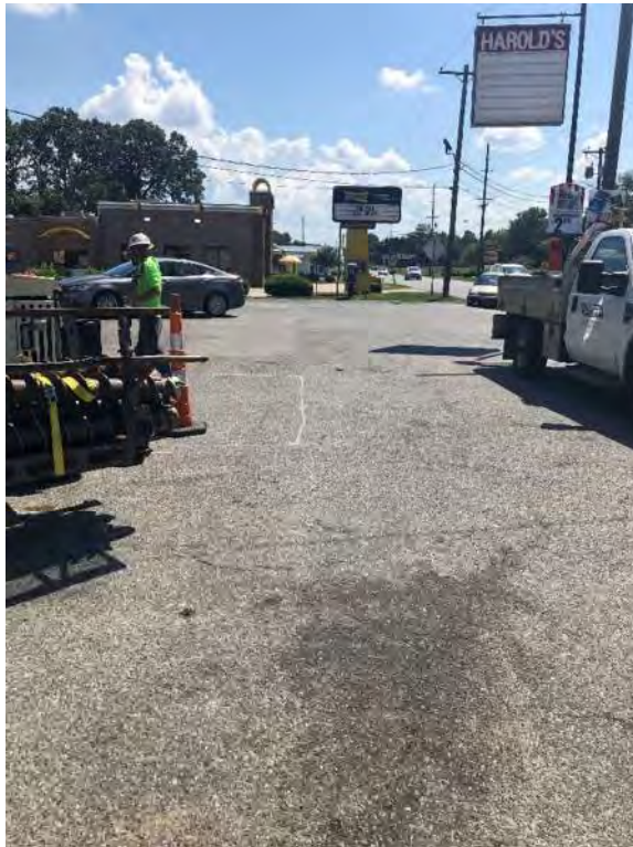
View facing southerly on Parcel 26 toward the four attempted borings which met resistance at 1.5-ft bgs.
