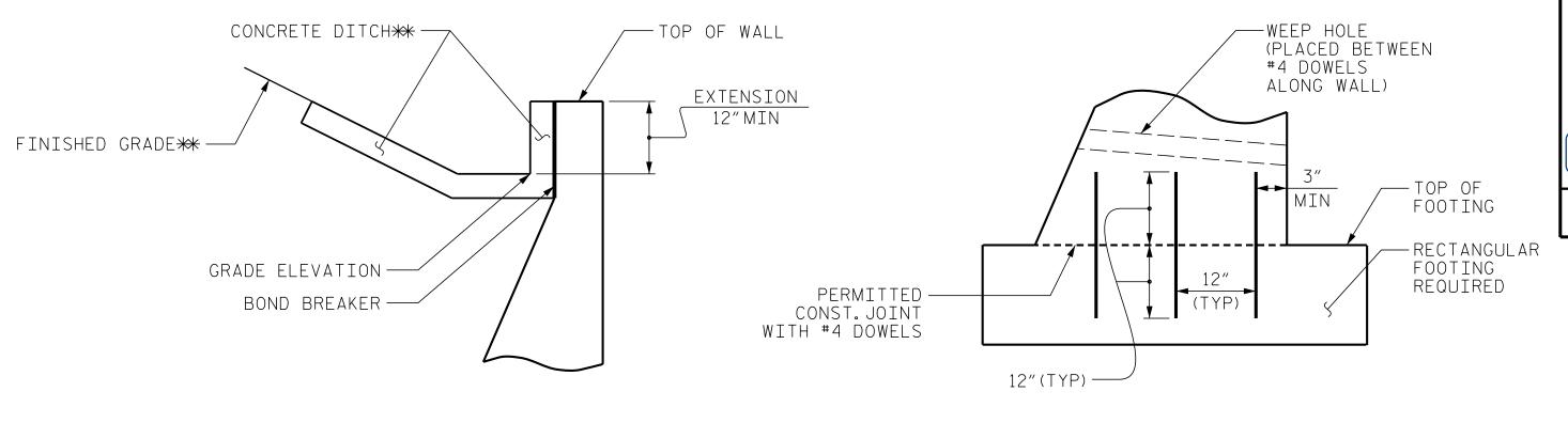
\*\*SEE ROADWAY PLANS FOR CONCRETE DITCH AND FINISHED GRADE DETAILS.
