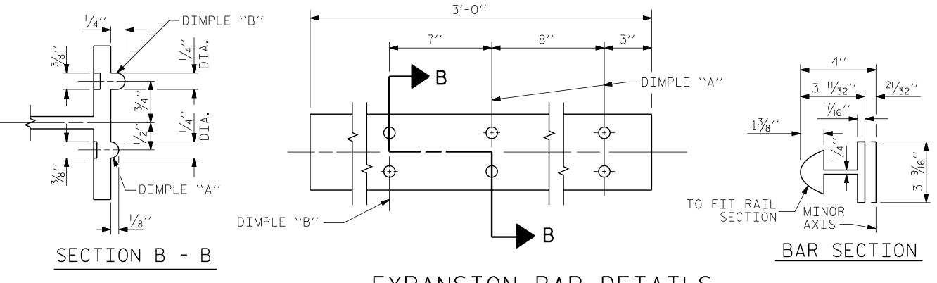
1/2" Ø [13 THREAD] HOLE FOR 1/2" Ø X 1" STAINLESS STEEL HEX HEAD CAP SCREW & 1/16" O.D., 17/32" I.D.,
