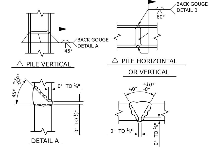
△ POSITION OF PILE DURING WELDING.
