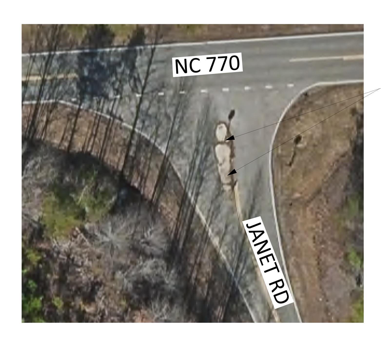
Relocate stop sign, in monolithic island, away from NC 770 and in line with stop sign on right shoulder of Janet Rd. New location should allow more room for trucks turning left onto NC 770 from Janet Rd.
