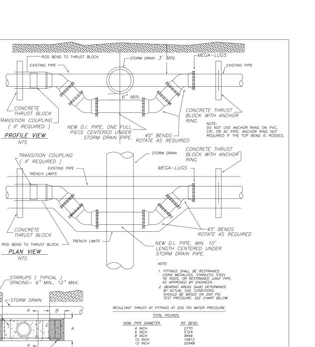
THE FOLLOWING OFTEN—USED SOIL VALUES FOR THE DEPTHS OF 4 FEET ARE LISTED ONLY AS A GUIDE\*. THE ENGINEER SHOULD SELECT THESE BEARING VALUES FOR EACH SOIL TYPE AND DEPTH OF COVER ENCOUNTERED ON THE SPECIFIC PIPELINE PROJECT. APPROPRIATE SAFETY FACTORS SHOULD BE APPLIED TO COVER FUTURE CHANGES IN PIPE DEPTH, SOIL BEARING CAPACITIES, ETC.
