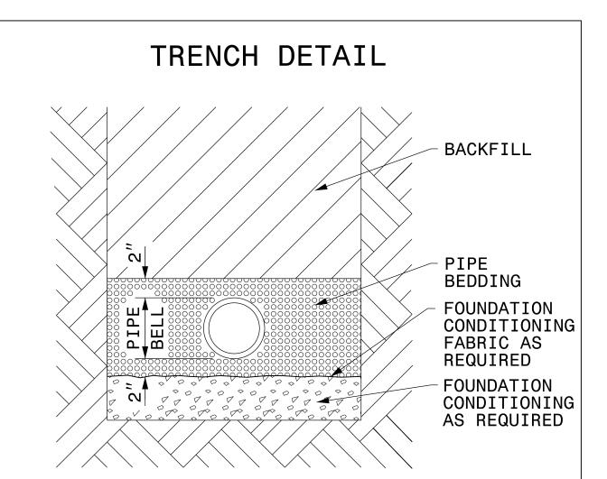
PLACE FOUNDATION CONDITIONING MATERIAL BELOW BEDDING IF REQUIRED, AS DIRECTED BY ENGINEER. PIPE BEDDED IN SELECT MATERIAL, CLASS II (TYPE 1) OR CLASS III. TRENCH BACKFILLED IN LOOSE 6" LAYERS COMPACTED TO TOP OF TRENCH USING LOCAL EXCAVATED MATERIAL IF APPROVED BY THE ENGINEER, OR SELECT MATERIAL. ALL MATERIAL SHALL BE FREE OF ROCKS, FOREIGN MATERIAL, AND FROZEN EARTH. COMPACTION SHALL BE TO APPROXIMATELY 95% DENSITY IN ACCORDANCE WITH AASHTO T-99 AS MODIFIED BY THE DEPARTMENT OF TRANSPORTATION.
