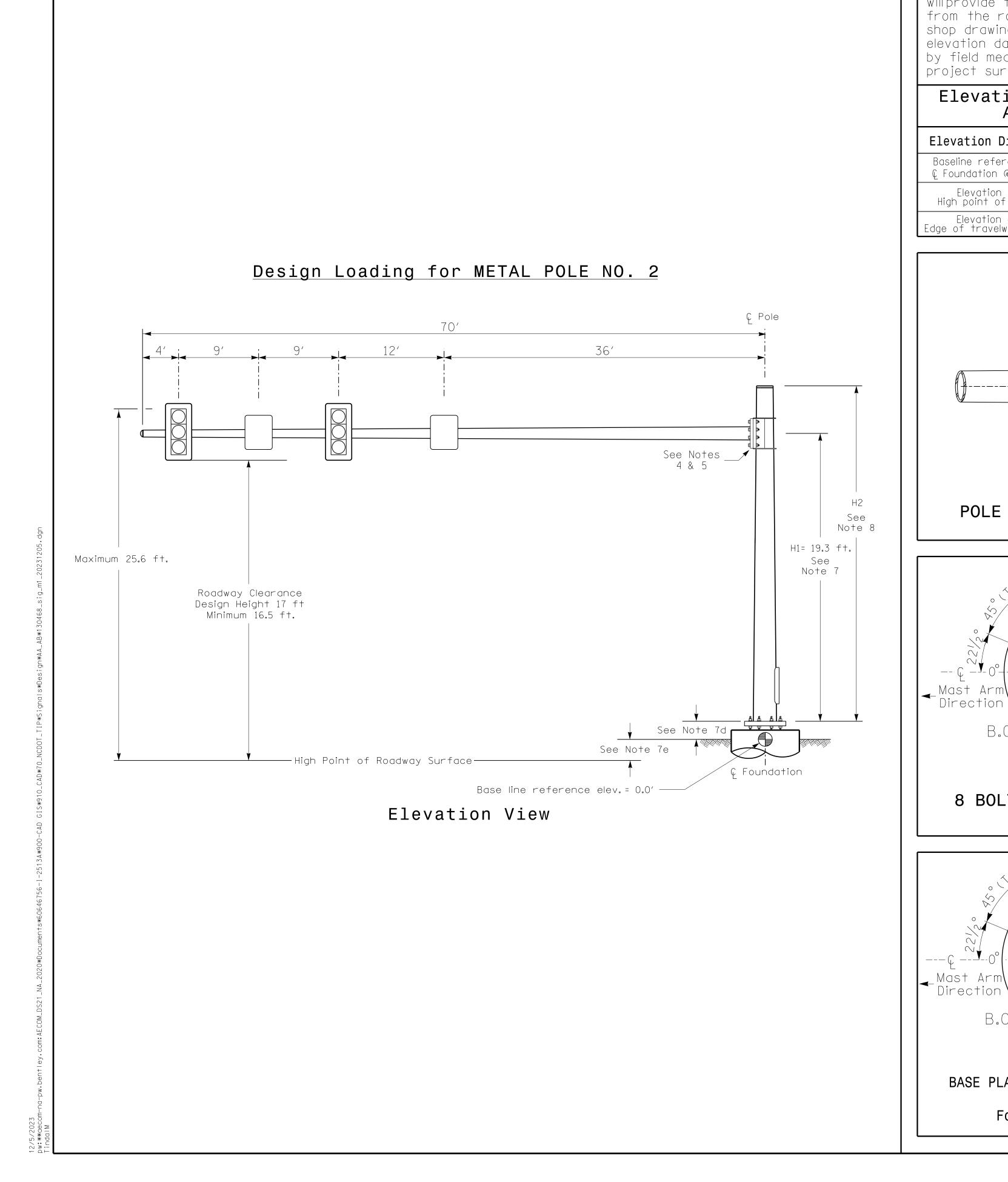
SPECIAL NOTE The contractor is responsible for verifying that the mast arm attachment height (H1) willprovide the "Design Height" clearance from the roadway before submitting final shop drawings for approval. Verify elevation data below which was obtained by field measurement or from available project survey data.
