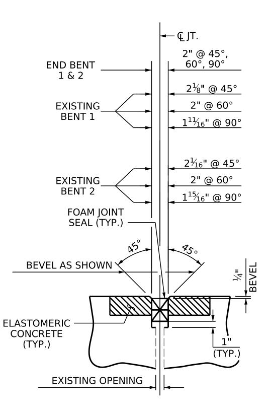
PROPOSED JOINT SEAL DETAIL
