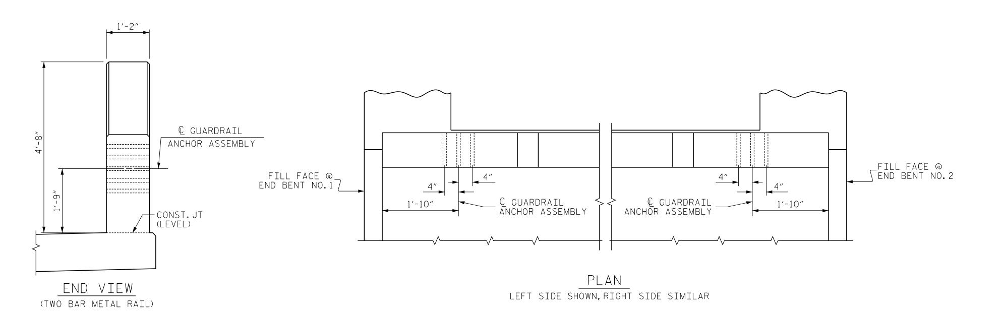
LOCATION OF GUARDRAIL ANCHOR AT END POST
