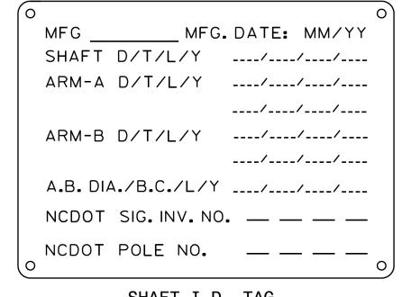
SHAFT I.D. TAG (PROVIDE ON SHAFT OF STRAIN POLES AND MAST ARM POLE SHAFT) ARM I.D. TAG
