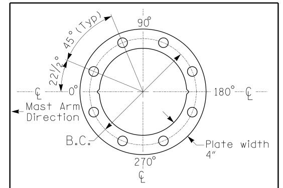
LOCK PLATE DETAIL For 8 Bolt Base Plate NCDOT Wind Zone 4 (90 mph)
