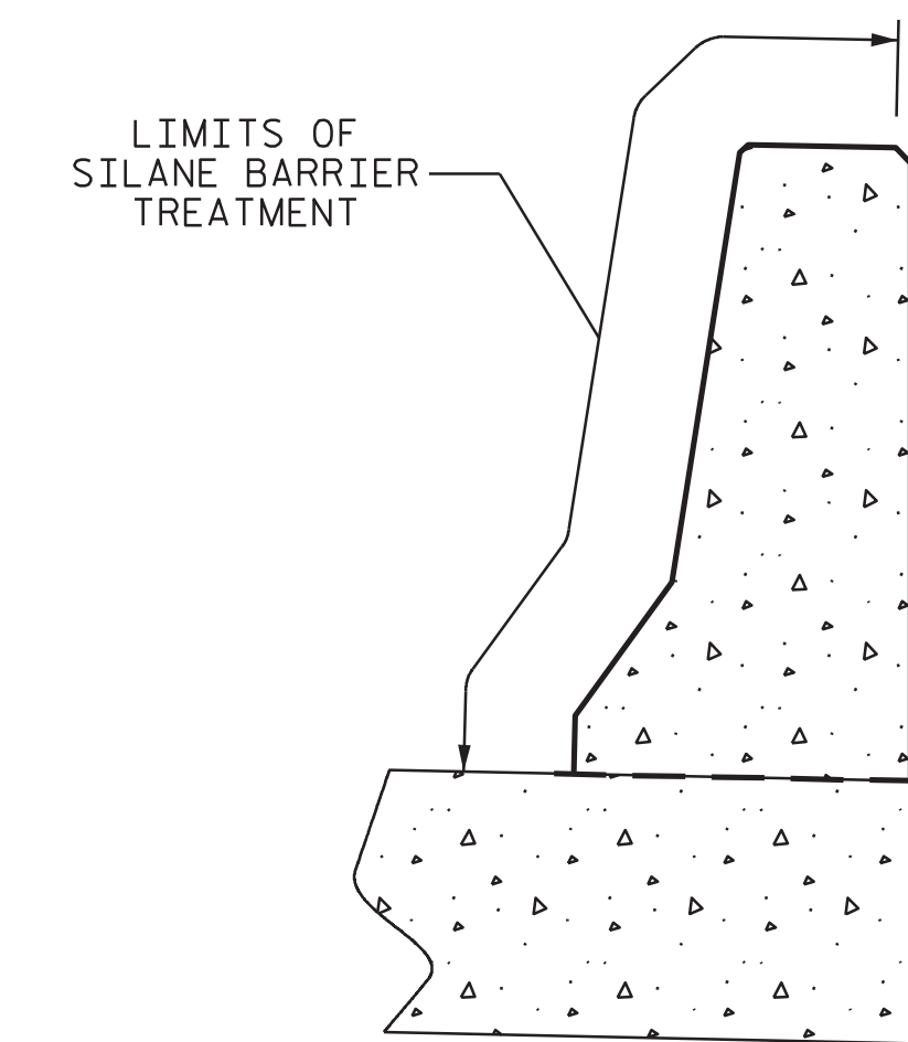
SILANE BARRIER RAIL TREATMENT
