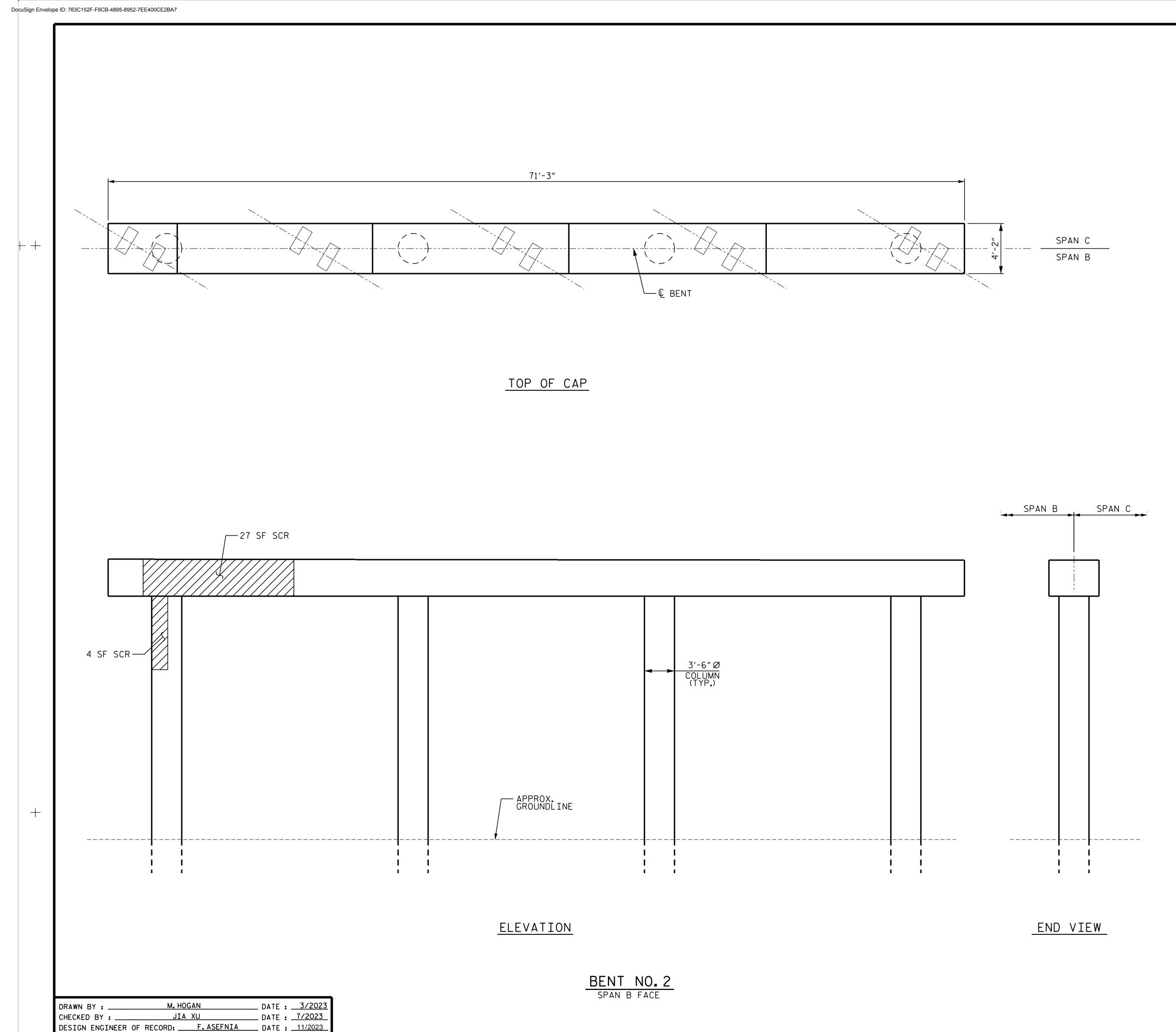
AS-BUILT REPAIR QUANTITY TABLE QUANTITIES BENT 2 SPAN B FACE ESTIMATE ACTUAL AREA SF ΛΟϔΠ̈́WE SHOTCRETE REPAIRS CAP 7.0 27.0 COLUMN 4.0 1.0 AOFÄWE лойпме CONCRETE REPAIRS CAP 0.0 0.0 EPOXY RESIN INJECTION LN.FT. LN.FT. 0.0 COLUMN 0.0 EPOXY COATING SQ.FT. SQ.FT. TOP OF BENT CAP 296.0
