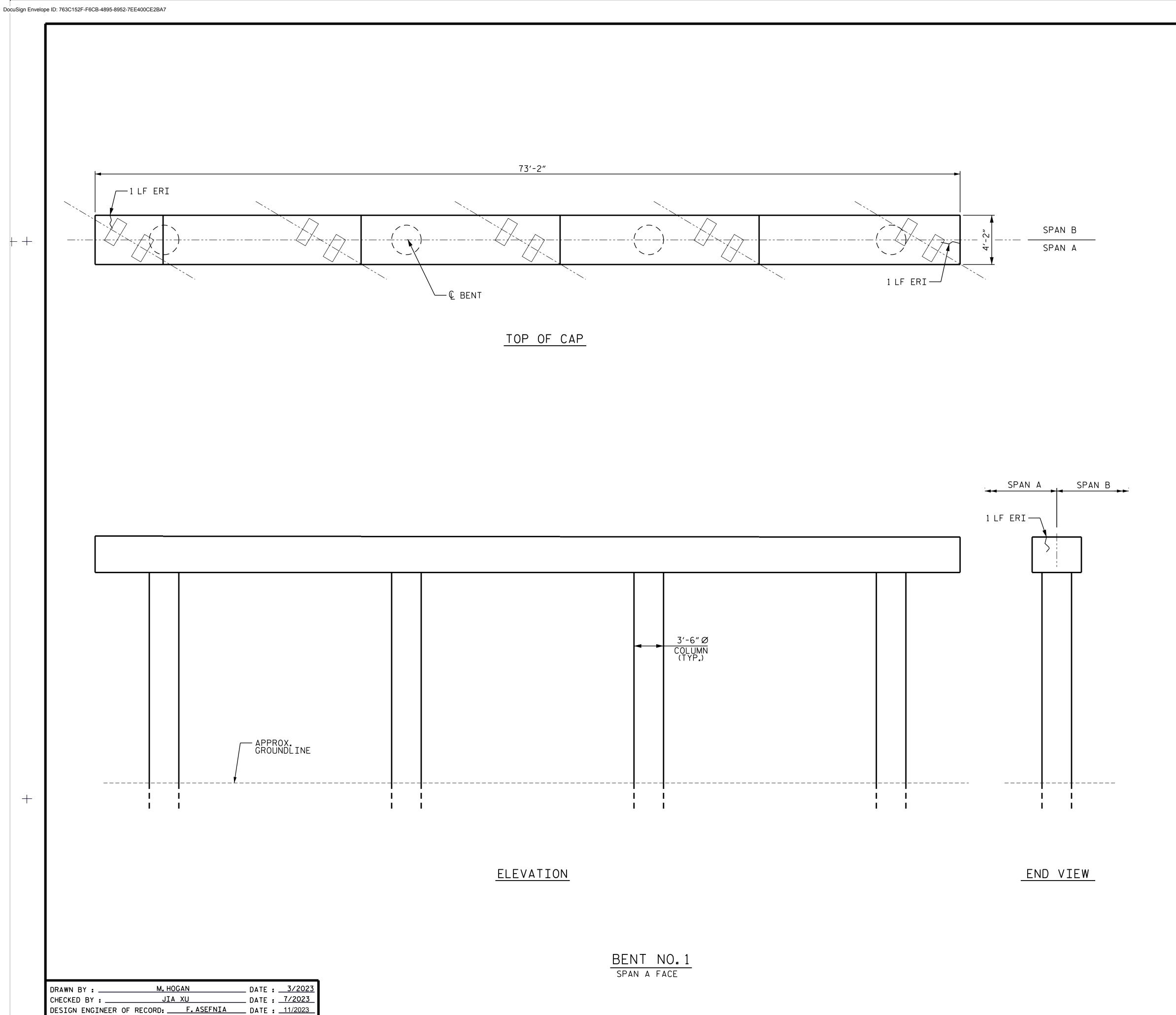
AS-BUILT REPAIR QUANTITY TABLE QUANTITIES BENT 1 SPAN A FACE ESTIMATE ACTUAL AREA SF **VOĽŪWE** SHOTCRETE REPAIRS CAP 0.0 0.0 COLUMN 0.0 0.0 AREA AOFÄWE лойпме CONCRETE REPAIRS CAP 0.0 0.0 EPOXY RESIN INJECTION LN.FT. LN.FT. CAP 3.0 COLUMN 0.0 EPOXY COATING SQ.FT. SQ.FT. TOP OF BENT CAP 295.0
