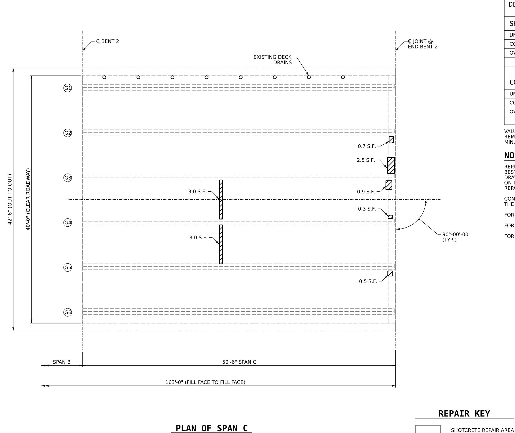
DECK UNDERSIDE REPAIR QUANTITY TABLE DECK UNDERSIDE REPAIRS SPAN C QUANTITIES ACTUAL **ESTIMATE** AREA VOLUME AREA VOLUME SHOTCRETE REPAIRS SF UNDERSIDE OF DECK 6.0 2.0 CONCRETE DIAPHRAGM 4.9 1.6 OVERHANG 0 AREA VOLUME VOLUME CONCRETE REPAIRS CF UNDERSIDE OF DECK 0 0 CONCRETE DIAPHRAGM **OVERHANG**
